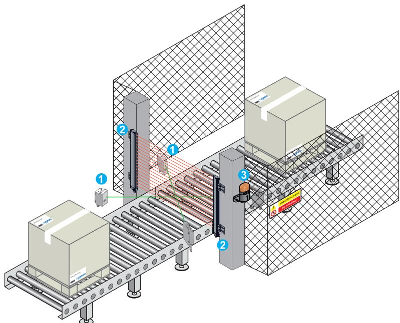
① Inhibition sensor (or muting sensor).
