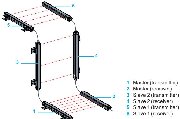
Multi-segments help protect multiple zones via a series connection. Only the first segment, known as the "master", is connected to the control cabinet or enclosure.
