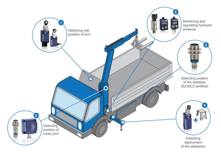
1 XCMV or XCMD Limit Switch Compact body and modular head allows easy mechanical adaptation.
